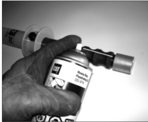
2. Drive bar thread protector. Keep threads clean and lubricated for easy installation of the optional 5 Pound Handle Weight.
